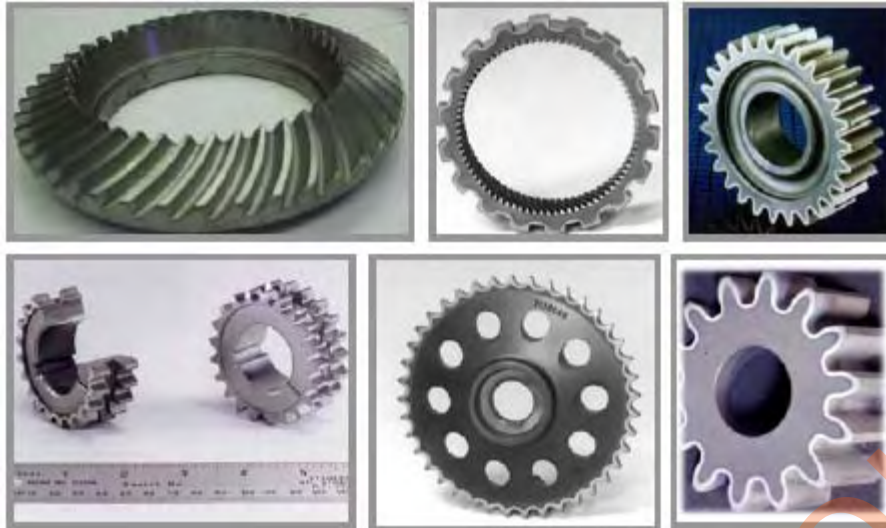
Figure 8. Examples of gears that use induction spin hardening techniques. Different patterns can be produced by properly controlling these parameters. Figure 9 shows a variety of induction-hardened patterns. They were produced by varying heating time, frequency, and power.
