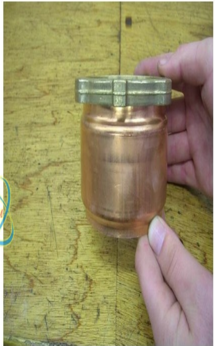
Brass ring and copper piece that will be soldered together for the 1 st step
